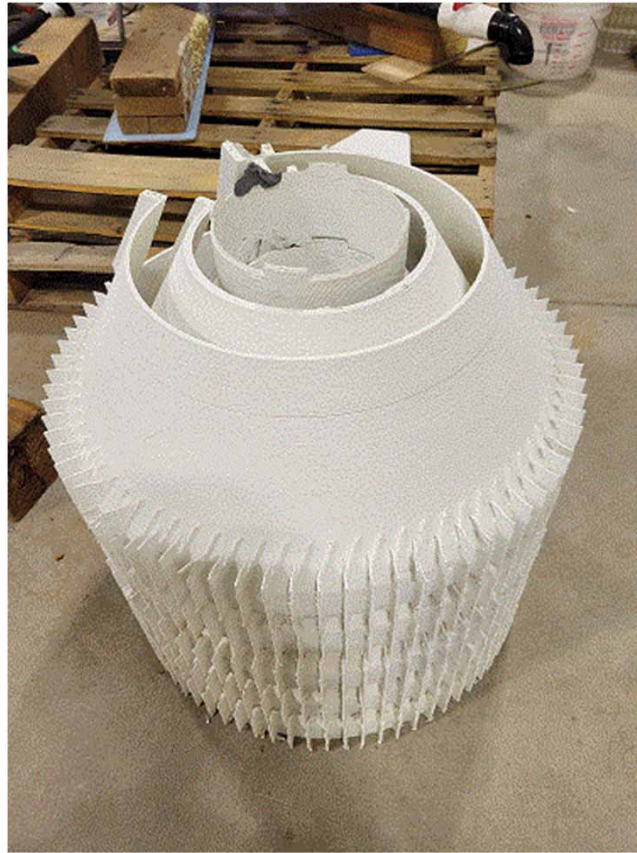
Figure 10 | A stack of smooth-surfaced cones (lamella cones).
