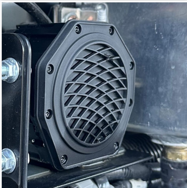
FIGURE 1 AVAS mounted on the MDEV.
