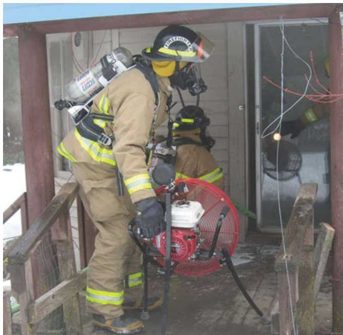
Figure 9: Fire fighter Operating SSI Fan (image courtesy fireapparatusmagazine.com) [121]
