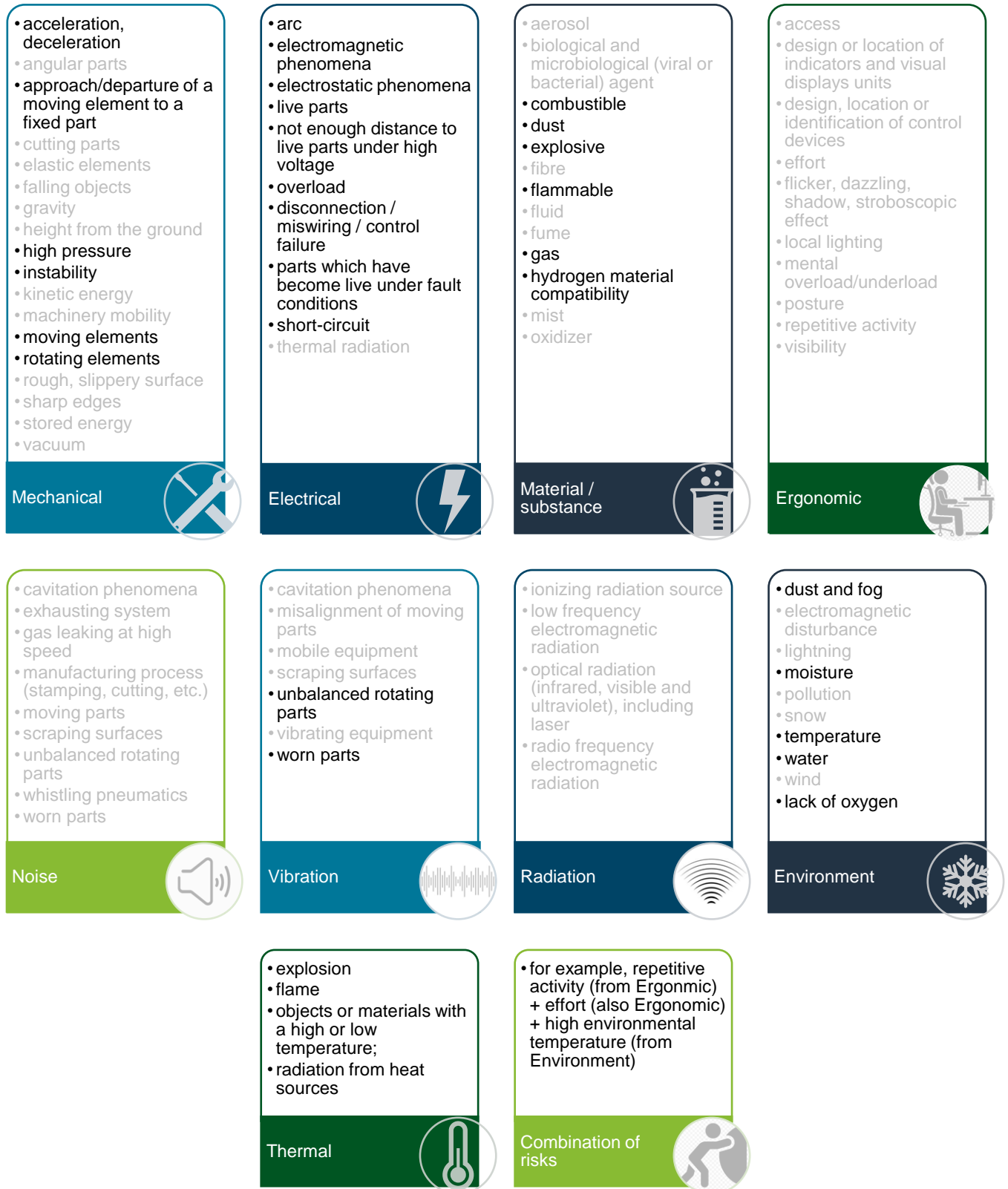
Figure 6: List of associated hazard groups and components. Light-grey font indicates hazards which were not identified in this risk assessment.
