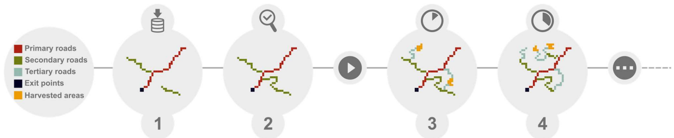
723 Figure 3 Diagrams showing the evolution of the forest road network simulated by the FRS module. Road 724 pixels are coloured according to their size category. (1) Input data is read by the module; (2) the roads
