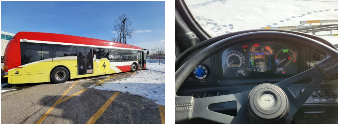
Figure 7: A Proterra electric bus (left) and operator dash board (right)
